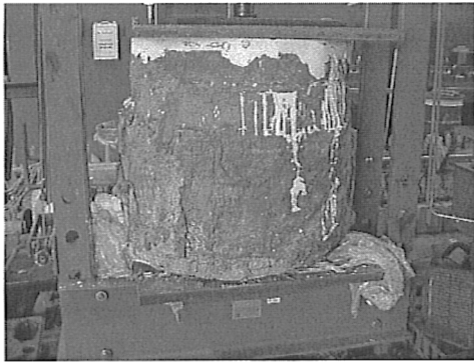
Figure 9 Full Scale Compression Test
