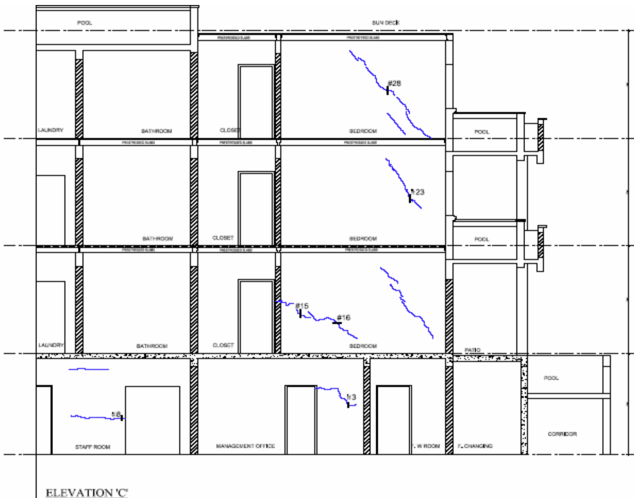
Figure 1 – Shear cracking ( \sim 45^\circ ) in east-west building walls.
