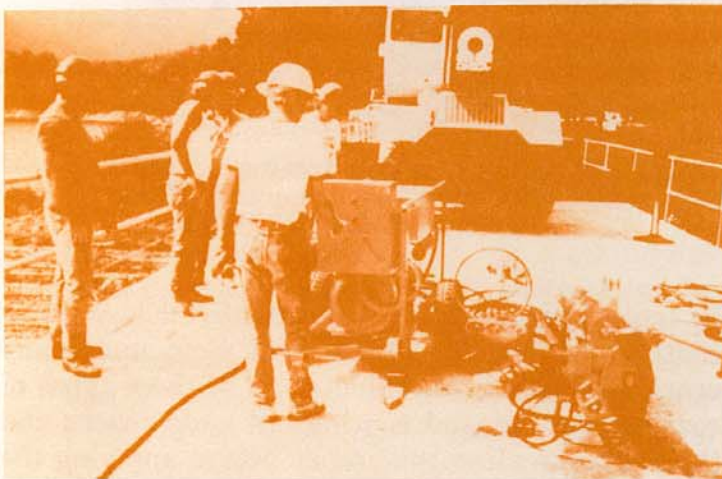
Figure 4. Components of the electrohydraulic coring rig (from right, mast w/head, controls, power pack)
