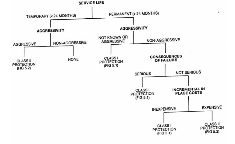
Figure 1. Corrosion protection decision tree (PTI, 1996).
