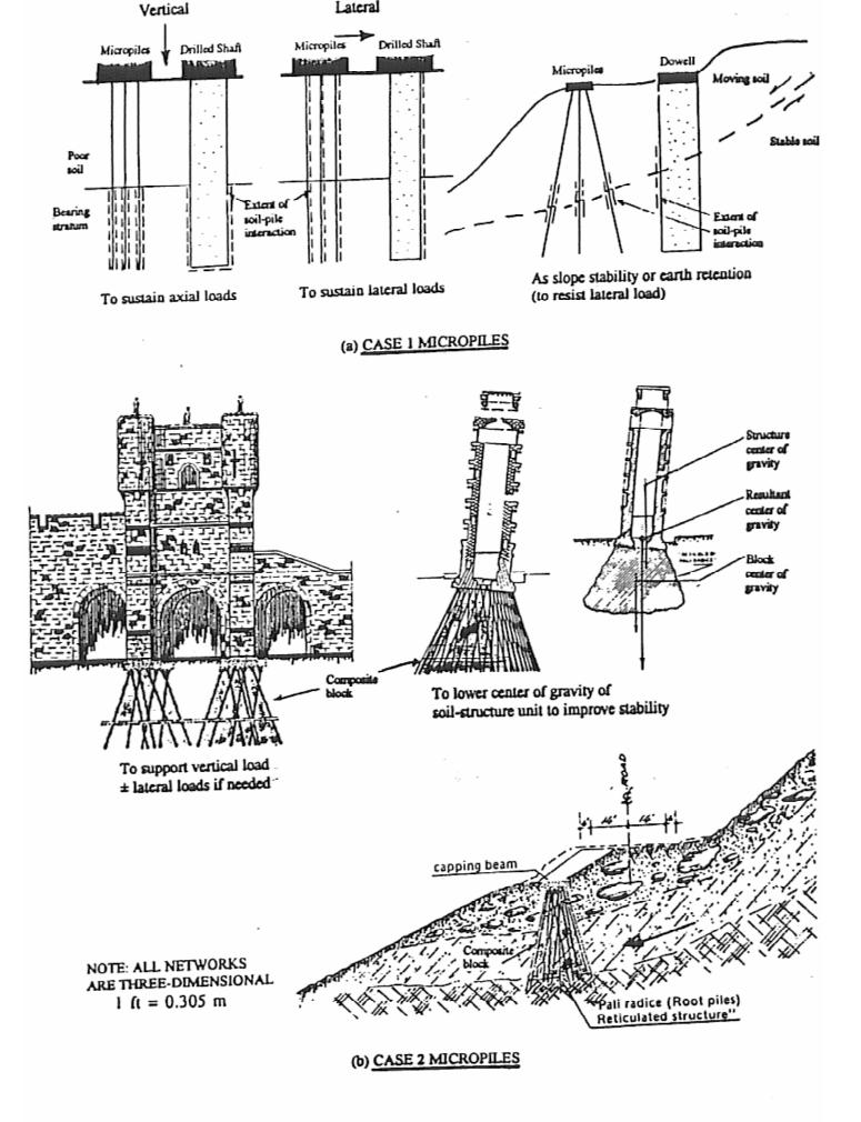
Figure 3. Fundamental classification of micropiles based on their supposed interaction with the soil.
