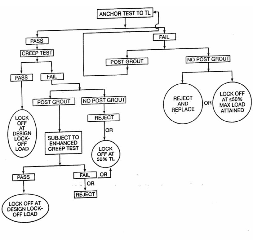
Figure 2. Decision diagram for acceptability testing of anchors (PTI, 1996).
